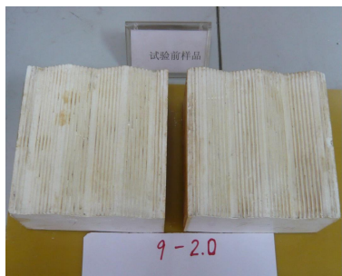
图 2 典型节理试件（二阶起伏体高 2 mm） Fig.2 Typical gypsum joint samples (second-order asperities of 2 mm height)
